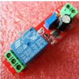
NE555 DC 5V Delay relay shield Timer Switch Adjustable Module $1.70
