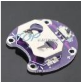
LilyPad Coin Cell Battery Holder CR2032 Battery Mount Module $1.62
