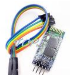
Wireless Serial 4 Pin Bluetooth RF Transceiver Module HC-06 $3.50
